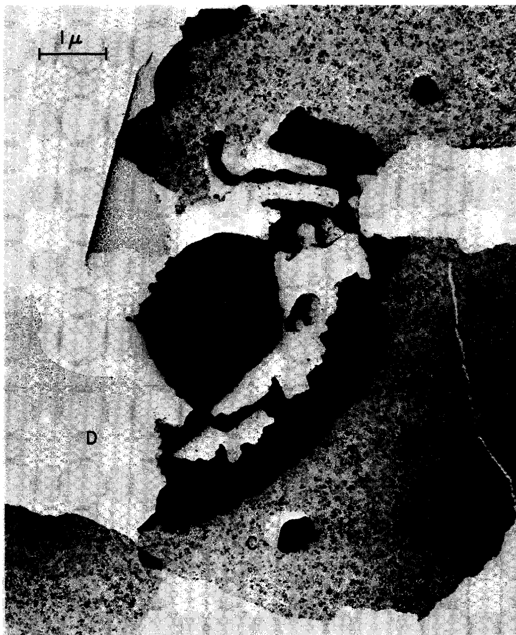
FIG. 1. Electron micrograph of a single-crystal compound (B) formed by interaction of Pt-Al alloy (A) with alumina substrate (C).
